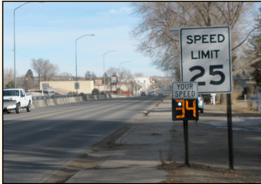
SPEED FEEDBACK SIGNS tell drivers their speed (measured by radar) and the speed limit on the road.
